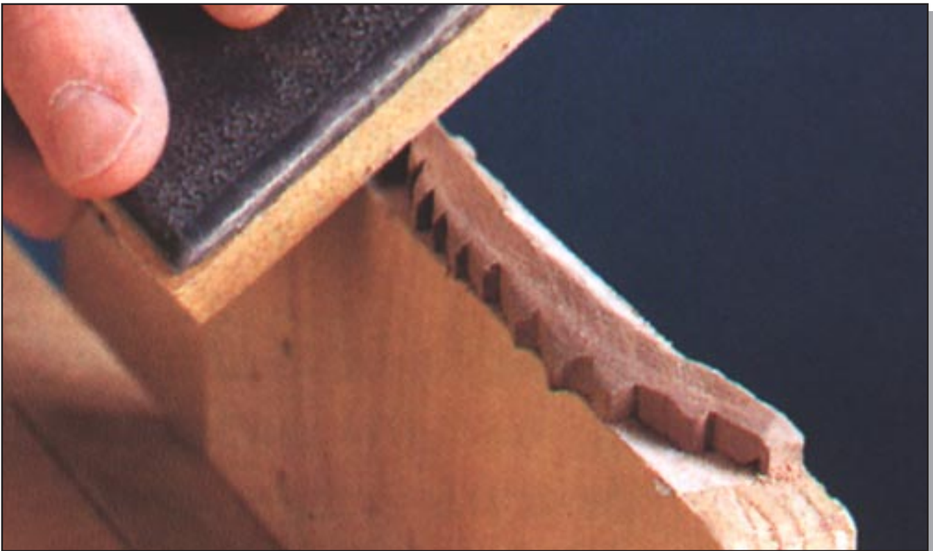
Use double-faced tape to secure a branch to the edge of \frac{1}{2} " or \frac{3}{4} " stock to steady the piece when shaping.
