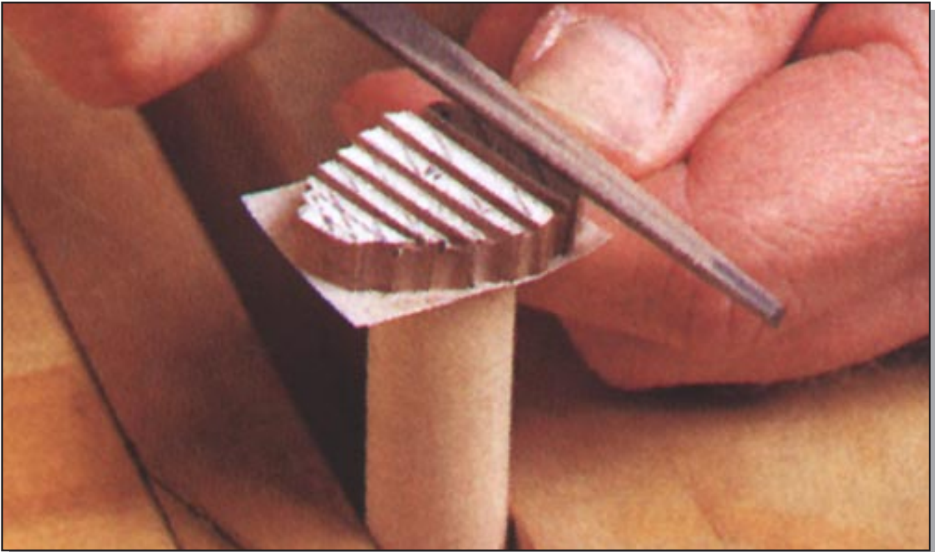
A 4"-long piece of \frac{5}{8} " dowel stock makes a sturdy handle for filing and sanding the pine cones to shape.
